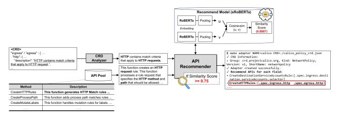
FIGURE 7. Example of the API recommendation process for generating a new adapter.
