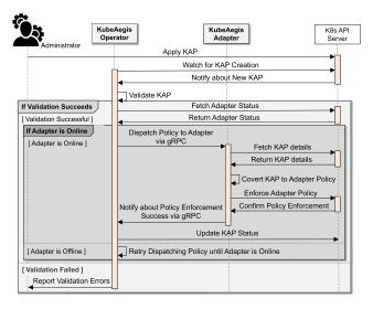
FIGURE 6. Sequence diagram for handling a KAP creation event.
