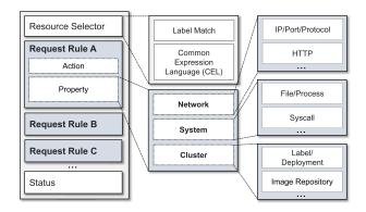
FIGURE 5. Partial views of KAP structure: The request rule involves network, system, and cluster properties.
