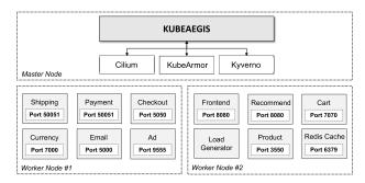
FIGURE 10. Overview of test environments: KubeAegis and three different adapters deployed on the master node.
