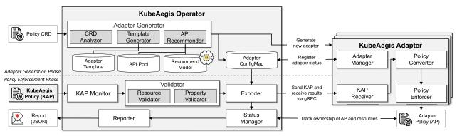
FIGURE 4. Overall architecture and workflow of KubeAegis with three key components: (i) KubeAegis Policy (KAP), (ii) KubeAegis Operator, and (iii) KubeAegis Adapter. Additionally, Our System Includes Two Operational Phases: Adapter Generation and Policy Enforcement.
